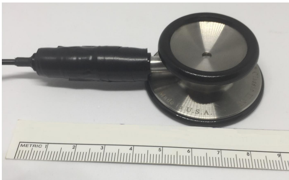
Fig. (2). The miniature electret microphone shown in Fig. (1) acoustically connected to a 3M Littman Classic II SE stethoscope head via a short piece of tubing.
